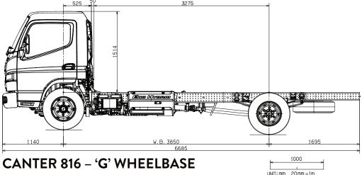
Scale = 1:50 (20mm = 1 metre). This scale is accurate when used on the original spec sheet, be aware that enlarging these illustrations can alter the scale and cause incorrect measurements. Fuso New Zealand and its authorised dealers always recommend customers seek professional advice from independent sources before commencing any engineering activities.
